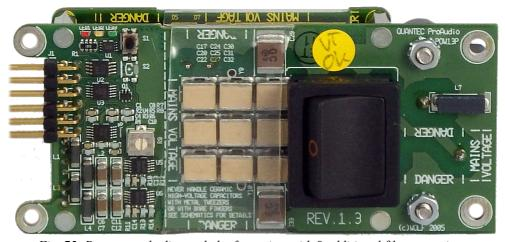
Fig. 75: Power supply dismantled – front view with 9 additional filter capacitors
